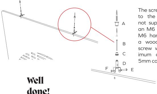
The screws for fixing to the ceiling are not supplied. Either an M6 set screw, a M6 hanger bolt or a wood chipboard screw with a maximum diameter of 5mm can be used.
